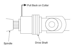
Figure 4-15 Disconnecting the Drive Shaft
